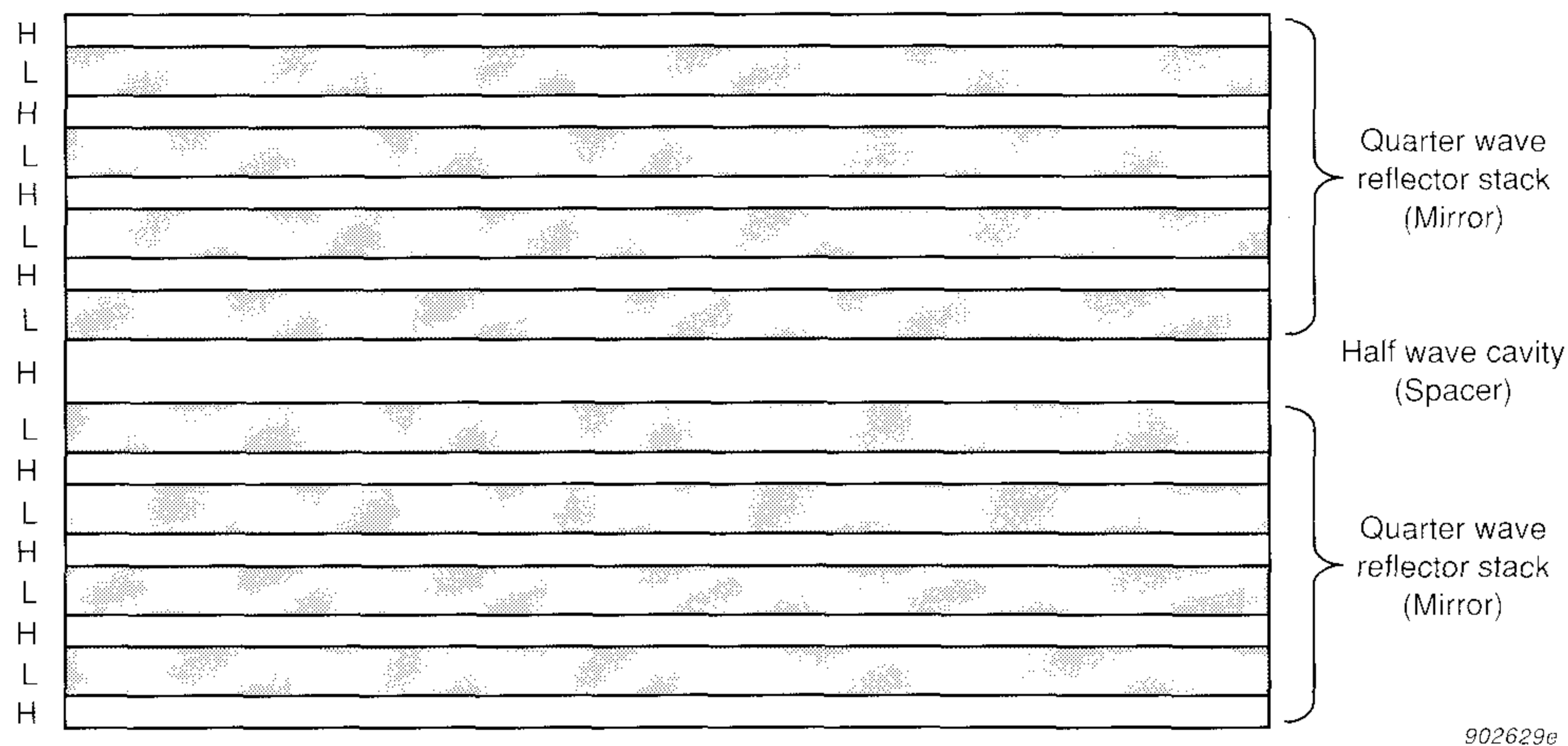
Fig. 6. Cross section of a typical "all-dielectric" single-cavity filter. L and H denote low and high refractive index respectively
